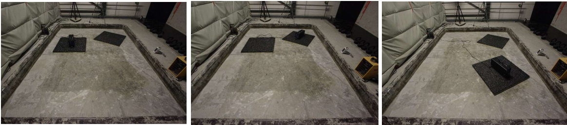
Photo test setup: Positions of the tapping machine on the testsample
