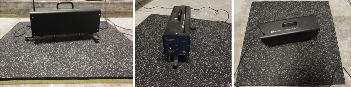
Photo: hammers of the tapping machine, impacting the testsample
